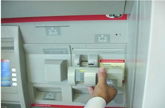
Figure 1: skimming device installed at card reader slot
