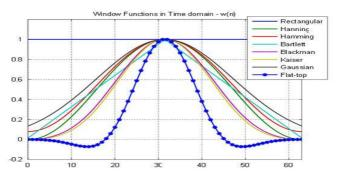
Fig 4: Different window functions in time domain
