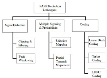
Fig. 2: Classification of PAPR reduction techniques
