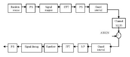
Fig.1 Block diagram of OFDM system
