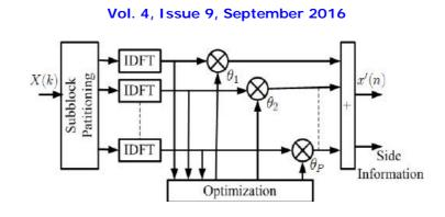
Fig. 6: Block Diagram of PTS Techniques [7]
