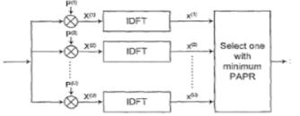
Fig 5: Block diagram of SLM technique [7]
