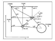
**Figure 1.** Localization by concurrent observation of several geometric beacons.
