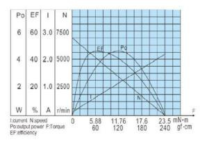
Figure 6. SPG30E-30K DC motor characteristics.
