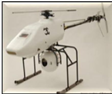
Figure 1: Prototype of aerial vehicle with a vision system attached below it.
