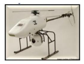
Figure 1.Prototype of an aerial vehicle with a vision system -camera attached below it.
