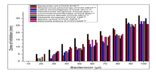
Figure 6. Minimum inhibitory concentration of bacteriocin indicated by the zone of inhibition.
