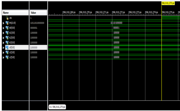
Fig 8. Simulation result for ROM data in cascade bi - rotation CORDIC
