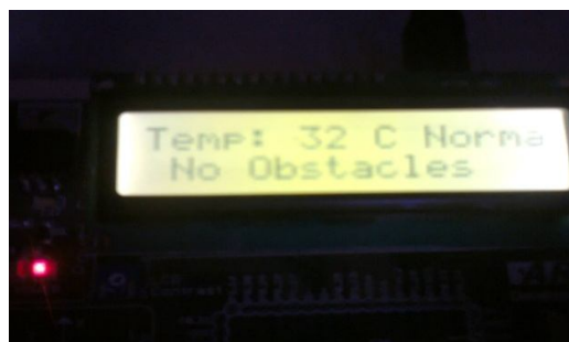
Fig5: IR and Temperature sensor interfacing with Arm7
