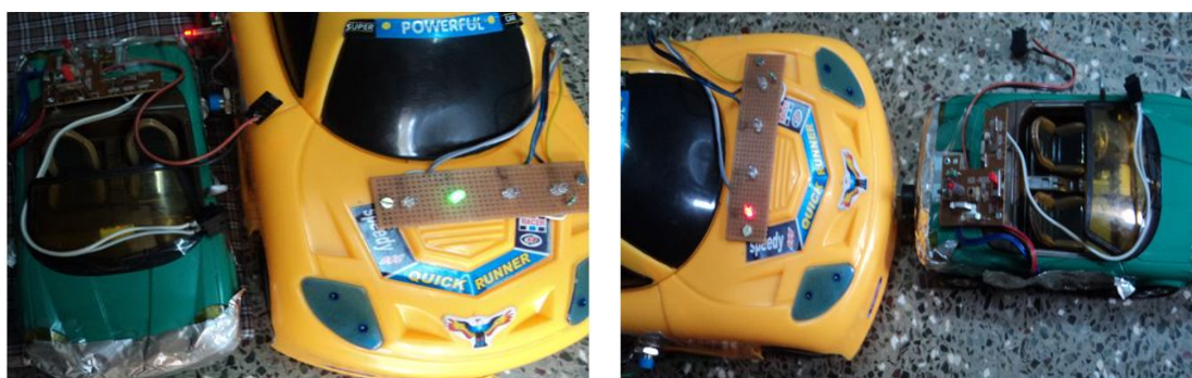
Fig: outputs of proximity sensors indicated through LED
