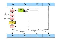
Fig 4. One MD5 operation. MD5 consists of 64 of these operations, grouped in four rounds of 16 operations. *F* is a nonlinear function; one function is used in each round.  $M_i$  denotes a 32-bit block of the message input, and  $K_i$  denotes a 32-bit constant, different for each operation.  $\leq \leq_s$  denotes a left bit rotation by *s* places; *s* varies for each operation.  $\blacksquare$  denotes addition modulo  $2^{32}$ .
