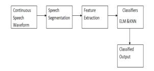
Figure 1. Block Diagram of Automatic speech Recognition
