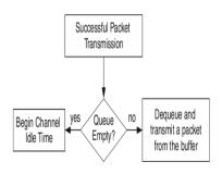
Fig 7.Successful Packet Transmission
