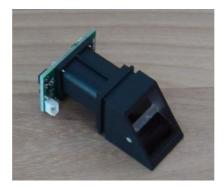
Fig. 4.R305 optical fingerprint scanner
