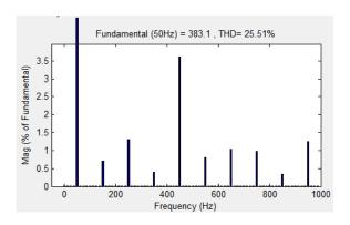
Figure 9. THD of three phase voltages
