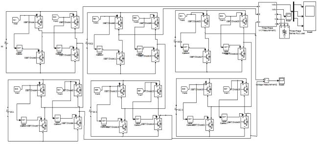
Figure 2.Three phase 5 level MLI
