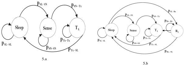
Fig 5 a:State transition diagram of a node acting as a Leaf node with transition probabilities in aWSN.
