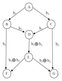
Fig 4: Encoding and Decoding operation of sensor node
