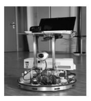
notebook screen. The video/audio communication between the telepresence robot and the subject's PC is done by means of commercial VoIP (Skype). This configuration allows the BMI user to interact remotely with people. For the sake of safety, the robot stops automatically in the case it loses the network connection with the BMI.
