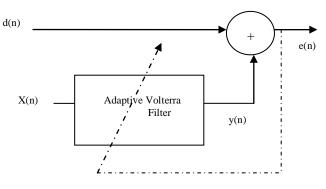
Figure.1 - A Block Diagram of Adaptive Volterra Filter
