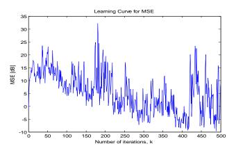
Figure.(a) The learning curve for the FIR system identification problem using LMS algorithm.
