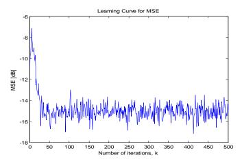
Figure.(b) The learning curve for the FIR system identification problem using RLS algorithm.
