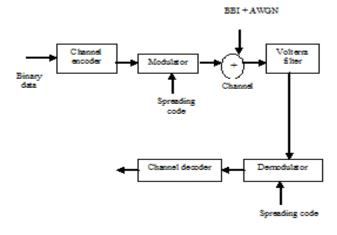
Figure.2 - Block Diagram of DSSS system along with Broadband interference introduced in the channel.
