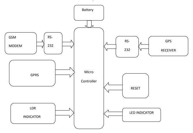
Fig.4 Automatic Broken Rail Detection Scheme using LED-LDR Assembly The proposed rail track detection system architecture consists of ARM7 controller, GPS, global system for mobile communications, LED-LDR Assembly, GPRS, DC Motor.
