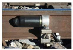
Fig.1 Ultrasonic Broken Rail Detector
