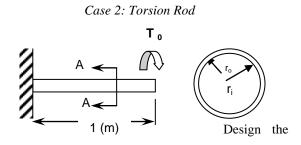
Section A-A, Outer radius -  $r_{\rm o}$ , Inner radius -ri Fig. 3 Torsion Rod
