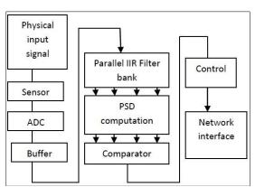
Fig. 5. WINS digital signal processing.
