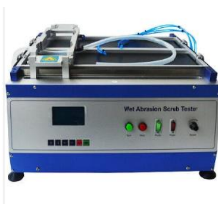
Figure 8. Sheen Scrub Tester used in the scrub resistance test for current acrylic paint formulation.
