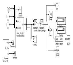
Fig 7 controller circuit of 12-pulse rectifier.
