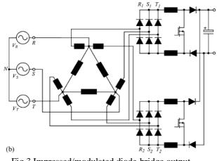
Fig 3.Impressed/modulated diode-bridge output
