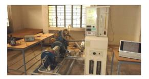
Fig.4: Experimental setup for combustion characteristics of CI-engine using Karanja biodiesel blends as fuel
