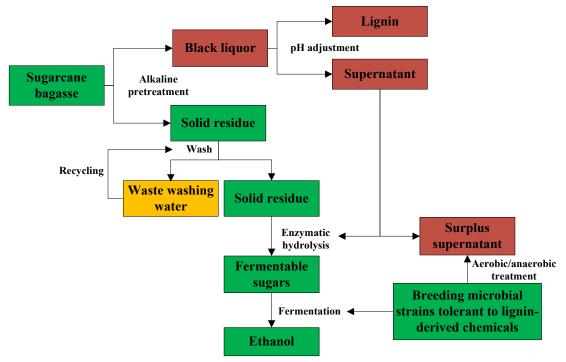
Figure 1. Prospective technical flow for cellulosic ethanol production based on alkaline pretreatment
