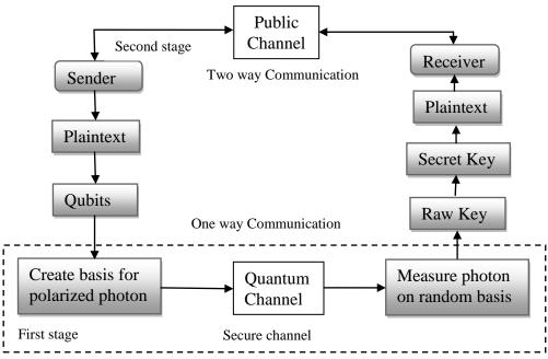
Fig.2. Quantum cryptographic communication system
