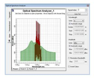
Figure 11: Unequal optical power spectrum (before optimization).
