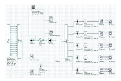
Figure 2: Schematic design of 16-channel WDM system for EDFA Length and pump power optimization.
