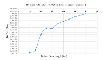
Figure 9: Characteristics of Bit Error Rate (BER) w.r.t optical fiber length for channel-1.
