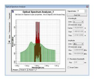
Figure 12: Flat output optical power spectrum (after GFF optimization).
