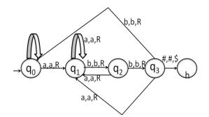
Figure 5: Turing machine for L
