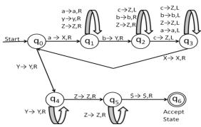
Figure 4: Transition diagram for  $\mathbf{L} = \{\mathbf{a}^{n}\mathbf{b}^{n}\mathbf{c}^{n} | \mathbf{n} \ge 0\}$
