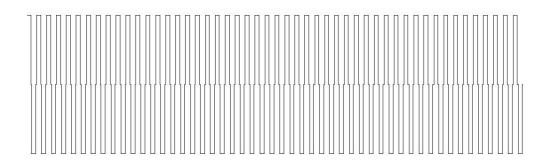
Fig.3Output Voltage Waveform Of Single Phase Three Level Cascaded H-Bridge Inverter.
