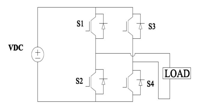
Fig 1 Single phase Three level cascaded H-Bridge inverter
