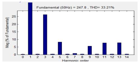
Fig 5THD of 3 level cascaded H-Bridge Inverter with RL load
