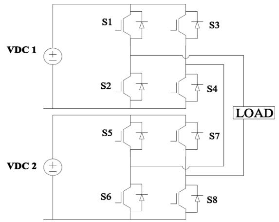
Fig 2 Single phase Five level cascaded H-Bridge inverter
