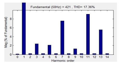
Fig 8THD Result For 5 Level Cascaded H- Bridge Inverter with RL load
