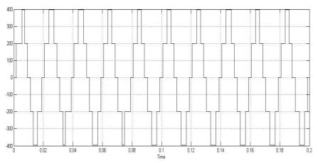
Fig.6 Output Voltage Waveform Of Single Phase 5 Level Cascaded H-Bridge Inverter.
