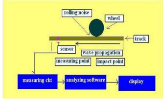
Fig.3 Measurement of rolling noise
