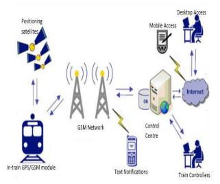
Fig. 1 GPS/GSM architecture
