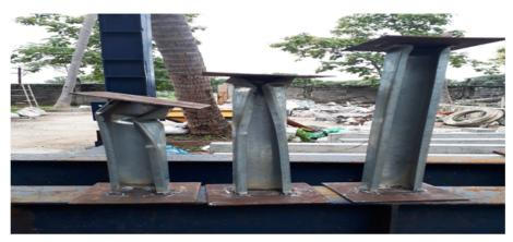
Figure 2: Channel sections of 400 mm, 500 mm and 600 mm lengths.
