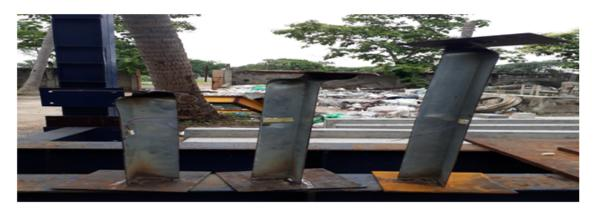
Figure 1. Angle sections of 400 mm, 500 mm and 600 mm lengths.
