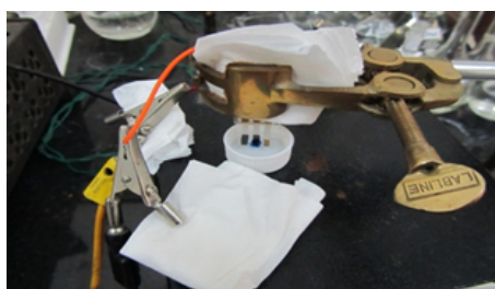
Figure 5b. Setup of biosensor for potentiostatic analysis.
