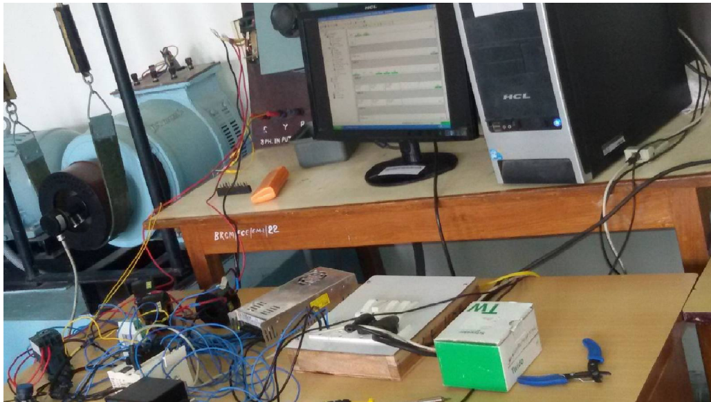
Figure 5: Hardware Connection of the Induction Motor Protection
