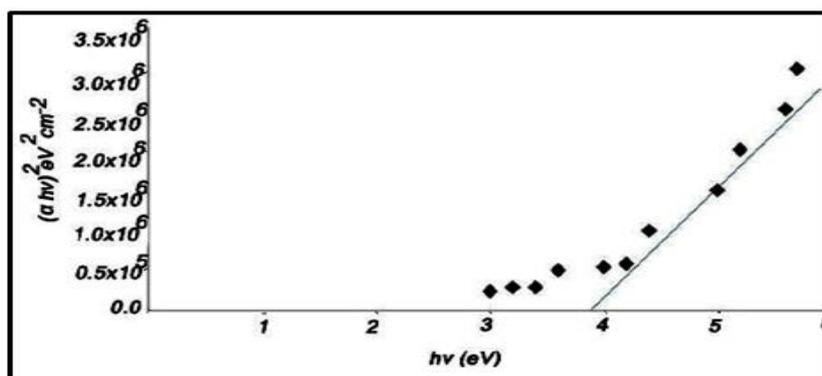
Figure 5. Tauc's plot of lithium ion and picric acid doped triphenyl phosphine oxide.
