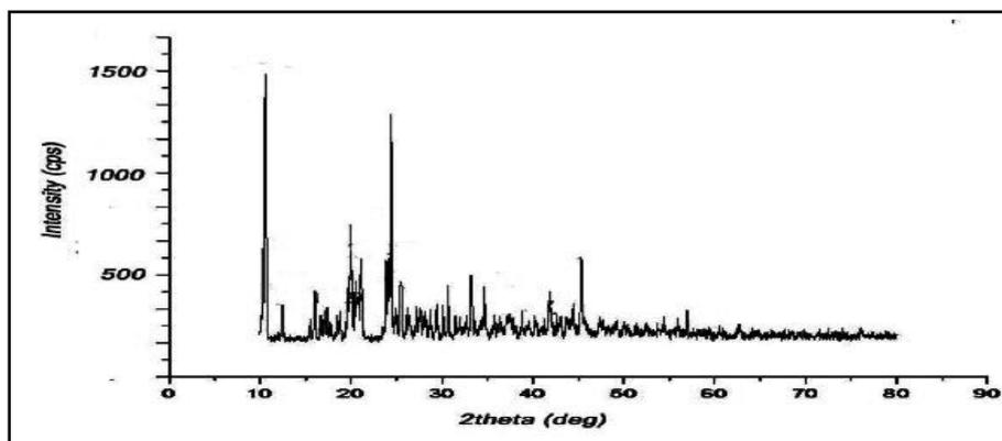
Figure 3. Powder X-ray diffractogram study of lithium ion and picric acid doped triphenyl phosphine oxide.
