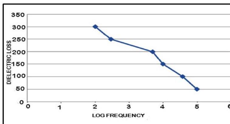
**Figure 9.** Variation of dielectric loss with respect to log frequency of lithium ion and picric acid doped triphenyl phosphine oxide crystals.
