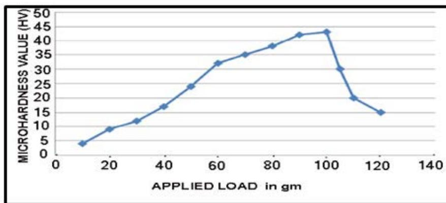
**Figure 7.** Micro hardness study of lithium ion and picric acid doped triphenyl phosphine oxide crystals.
