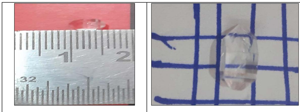
**Figure 2.** The as grown crystal of lithium ion and picric acid doped triphenyl phosphine oxide.
