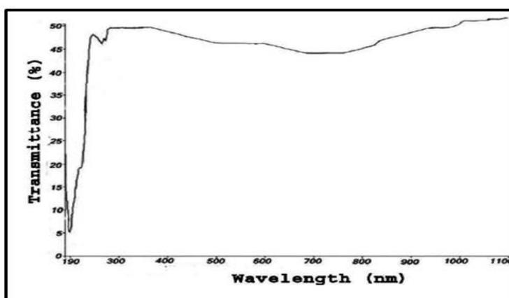
Figure 4. UV-vis-NIR studies of lithium ion and picric acid doped triphenyl phosphine oxide crystal.
