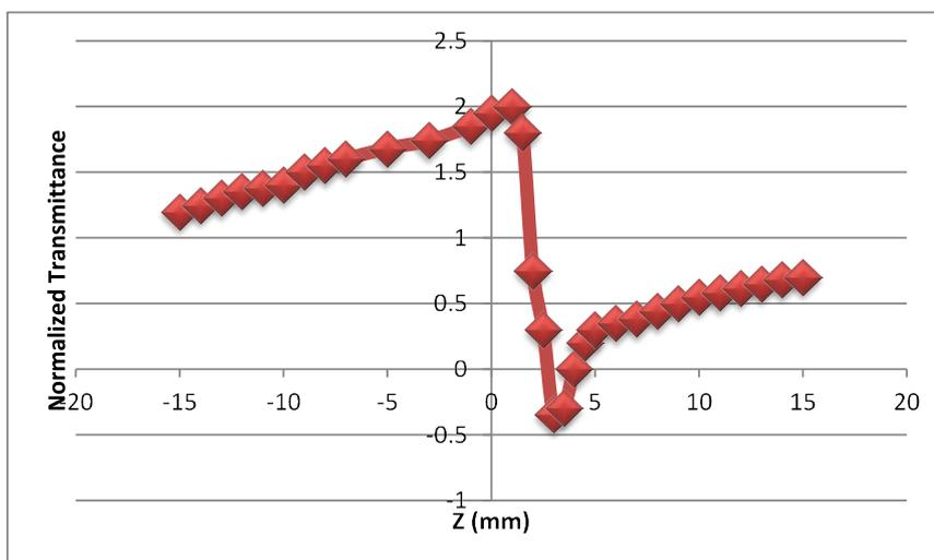
**Figure 6.** Z-scan studies of lithium ion and picric acid doped triphenyl phosphine oxide.
