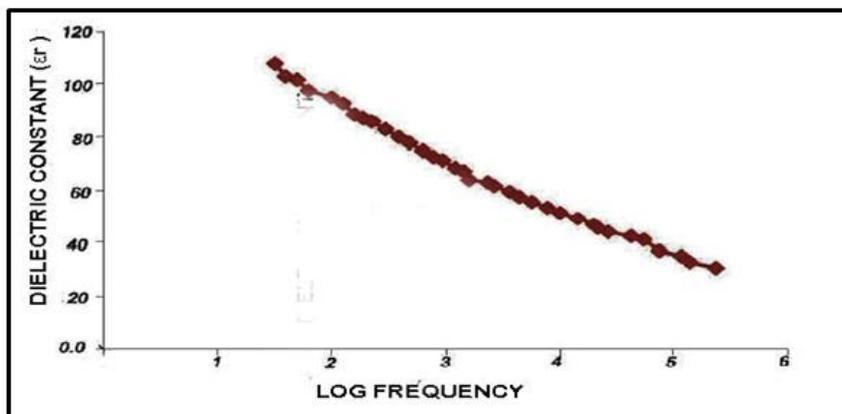
**Figure 8.** Variation of dielectric constant with respect to log frequency of lithium ion and picric acid doped triphenyl phosphine oxide crystals.
