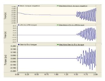
Fig.5. Oscillation at Generator to exciter torque is increased at resistance  $6.0832\Omega$ .
