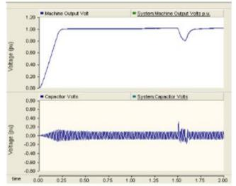
Fig.6. Oscillation at the output and capacitor voltage is decreased at resistance  $95\Omega$ .
