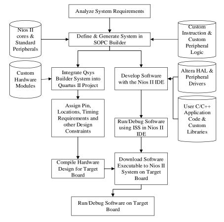
Fig. 3 Hardware & Software Codesign [16]
