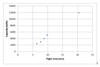
Figure 4: Flight times with various battery sizes.
