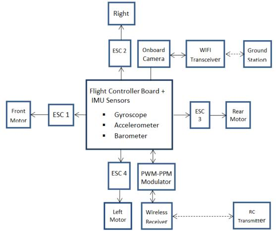
Figure1: Block diagram of the Quadcopter.
