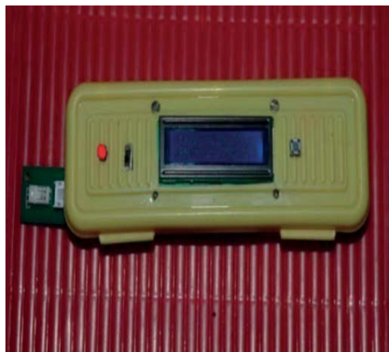
Figure 7: Photograph of relative humidity and temperature measurement system.
