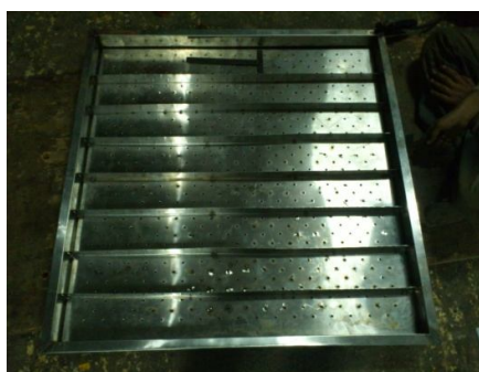
Figure 3: Actual photo of adsorbent bed
