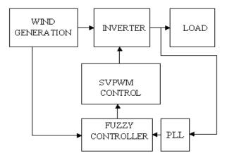
Fig.3. Block Diagram of Proposed System
