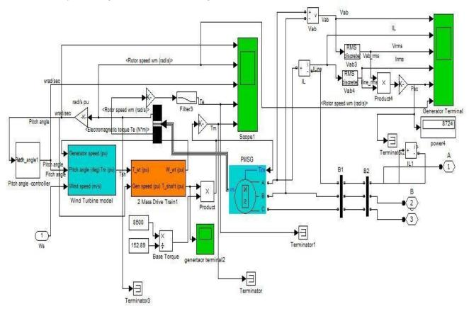
Fig.5 Simulink Diagram of Wind Generation Block
