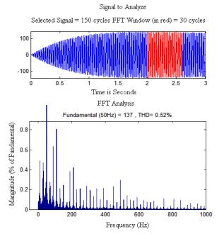
Fig.10 FFT Analysis of Harmonics Level in Output
