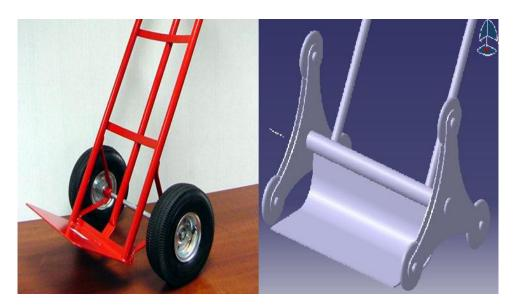
Figure 1: Initial design of Roller based wheel arrangement and wheel frame
