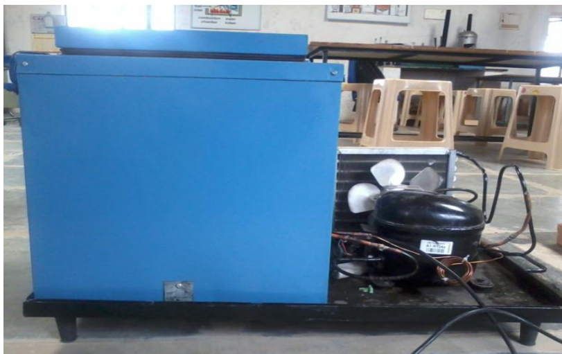
Figure 5: Fabricated Geometry of cold storage
