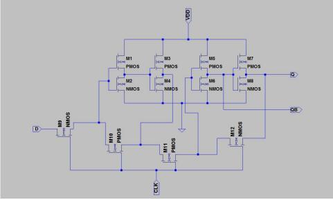
Fig. 3: DFF using Pass Transistor Logic (PTL)
