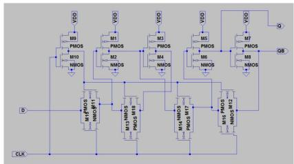
Fig. 3: DFF using Transmission gate Logic(TG)
