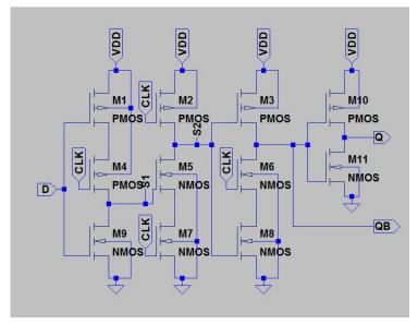
Fig. 2: D-flip-flop using TSPC Logic
