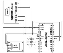
Fig. 6: Schematic Diagram of the GPS, GSM/GPRS Module and the Microcontroller.
