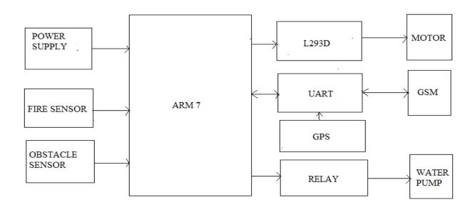
Fig: 1 Block diagram of supervising robot using GSM Module
