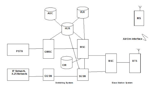
Fig: 2 Block diagram GSM-GPS Architecture
