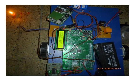
Fig: 5 Controllers displaying the fire detection and the message has been sent
