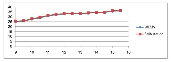
Fig. 9 Temperature comparison between WEMS and SMA sensors on 26/1/2015 since 09 AM to 03:30 PM
