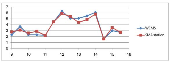
Fig. 13 Wind speed comparison between WEMS and SMA sensors on 26/1/2015 since 09 AM to 03:30 PM
