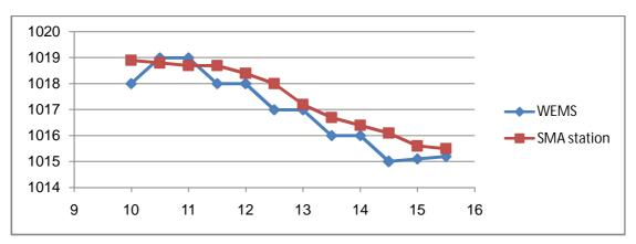
Fig. 5 Pressure comparison between WEMS and SMA sensors on 13/1/2015 since 10 AM to 03:30 PM
