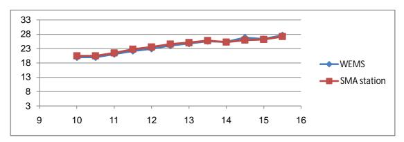
Fig.4 Temperature comparison between WEMS and SMA sensors on 13/1/2015 since 10 AM to 03:30 PM
