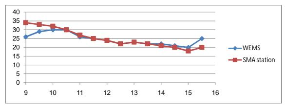
Fig. 11 Humidity comparison between WEMS and SMA sensors on 26/1/2015 since 09 AM to 03:30 PM
