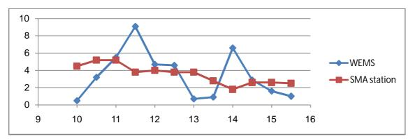
Fig. 8Wind speed comparison between WEMS and SMA sensors on 13/1/2015 since 10 AM to 03:30 PM
