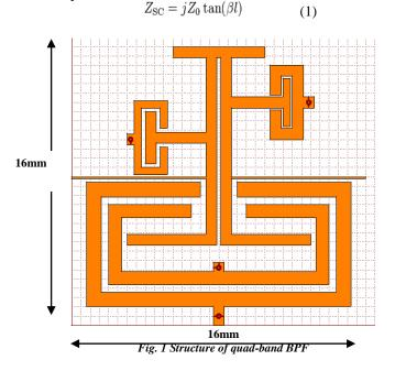
Any value of reactance can be made, as stub length is varied from zero to half a wavelength. Four shorted stubs are attached with each of the resonator. The stubs are shorted for the frequency selective operations over the LTE frequency bands. The size of the circuit is  $16 \times 16$ mm. FR4 is used as the substrate with 4.4 as dielectric constant ( $\varepsilon$ r). The distance between the resonator and the feed line is 0.2mm.
