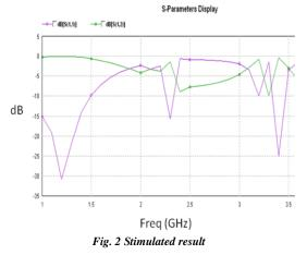
The resultant bands can be used for many wireless applications. This provides huge advantage for this design. The insertion loss obtained is at 0dB and return loss has maximum dip at -32dB.
