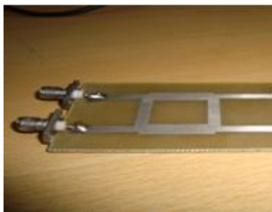
Fig.5 Photograph of a hybrid coupler with FR4 dielectric
