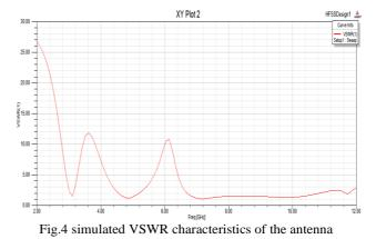
At the notch frequency, the current flows are more dominant around the parasitic element, and they are directed oppositely between the parasitic element and the radiation patch. As a result, the desired high attenuation near the notch frequency can be produced. The generated notched bands avoid interference at the existing WiMAX and WLAN applications.
