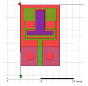
Fig.1 Design structure of proposed antenna.
