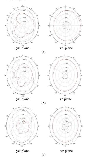
Fig.6 Radiation patterns of the antenna. (a).3.1GHz, (b).4.8GHz and (c) 7.2 GHz.
