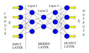
Figure 2: Generalized Structure of Multi Layer Perceptron (MLP) Neural Network Model
