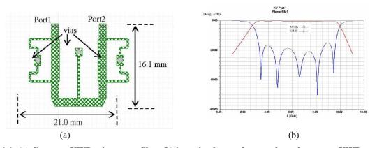
Fig 1.1: (a) Compact UWB microwave filter (b) insertion loss and return loss of compact UWB microwave filter
