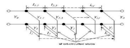
Fig1.3: short circuited stubs filter model
